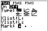
4. Turn on the plot by highlighting **ON** and pressing **ENTER**, then highlight the histogram chart (with the bars) and press enter, then enter the appropriate lists into **Xlist** and **Ylist**. The independent variable (the variable we are studying) will always be shown as the Xlist and the frequency will always be shown as the Ylist.
